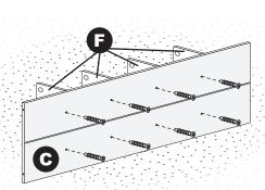
Install the four Upper Shelf Dividers (F) to the Upper Shelf Panel (C) with eight Hex Screws (L) using the Hex Tool.
