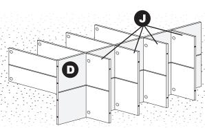
Place two Cam Locks (M2) into the recessed holes on each Lower Shelf Divider (J), with the arrow facing the closest edge.
