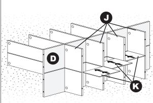
Slide three Lower Shelf Backs (K) into the grooves on the **Lower** Shelf Dividers (J) as shown, until fully seated into the groove on the underside of the Lower Shelf Panel (D).
