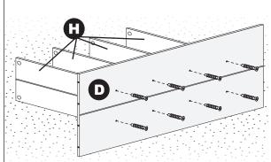
Install the four Locker Dividers (H) to the Lower Shelf Panel (D) with eight **Hex Screws (L)** using the Hex
