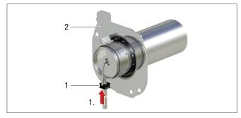
Push on the fuel connection grommet (1). Bottom edge of the grommet is flush with the combustion chamber flange (2).
