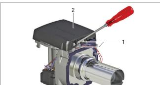
• Unlock the snap connections (1) on the blower cover (2) and remove the blower cover.
