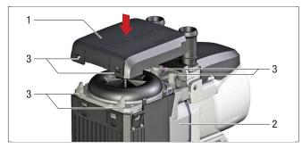
Place the blower cover (1) on the blower housing (2) and push downwards, until the snap connections (3) latch into position.
