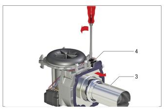
Pull the combustion chamber (3) together with the glow plug off the blower housing.
