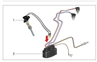
After replacing the glow plug (1) or lead harness of the heater (2), plug the glow plug connection cables onto connector -XB4 in chamber 3 and 4.
