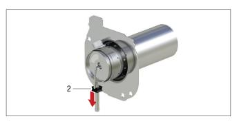
• Pull off the fuel connection grommet (2) from underneath.
