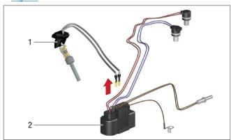
• Unplug the WH connection cables from the glow plug (1) at the connector -XB4 (2) (chamber 3 and 4).
