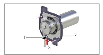
Hold both seal parts together and push them upwards between the combustion chamber flange (2) and the fuel connection grommet (1). The drillholes in the seal and combustion chamber lie above each other.
