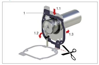
• Remove the seal (1) from the combustion chamber.
