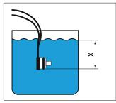
The sensor test is performed in liquid at temperatures up to max. 200 °C.
