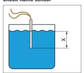
The sensor test is performed in liquid at temperatures up to max. 200 °C.
