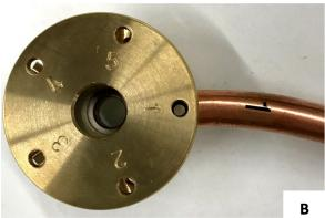
Lock the stem to the hub using provided spring washers and screws. Screw in manually as tight as possible Fig. C, DO NOT USE POWER TOOL!
