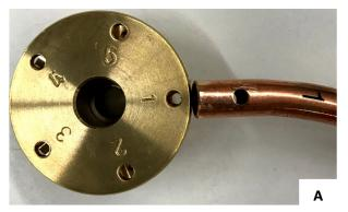
Align the hole on the stem with the hole on the hub Fig. B.
