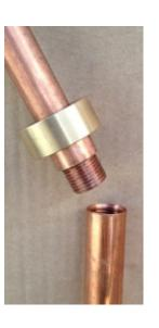
STEP 10. Slide the outer tubing to the inner tubing.
