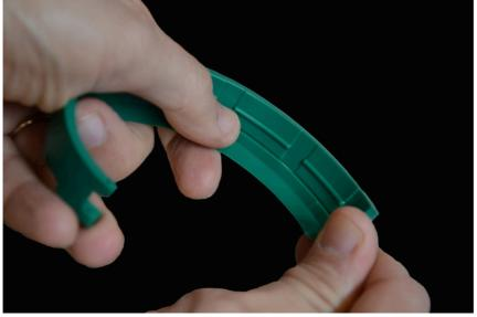
4. Push to join the two scraper's extremities. While contacting the extremities, slide down from the upper hole the included cotter pin (top-down).
