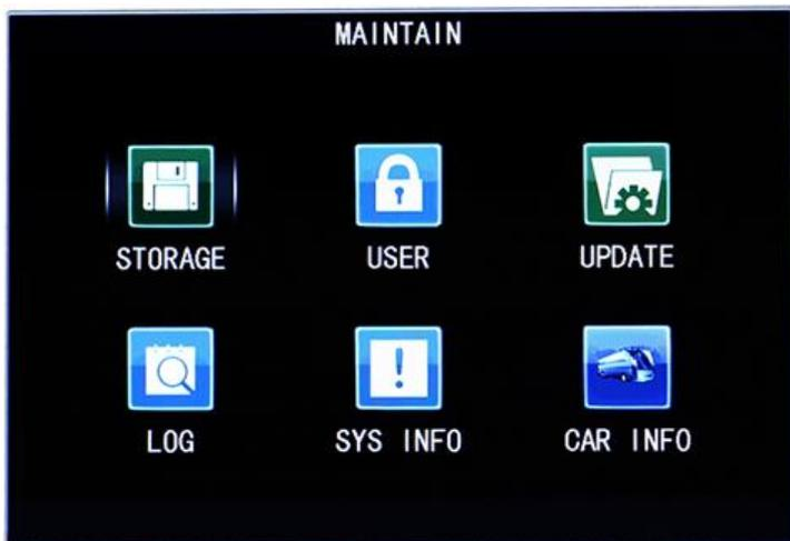
4.11 Storage Management; View the current device capacity, available capacity, and whether to format all the data within the device
