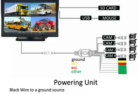
Tie dc+ wire and acc wire together and connect to a power source
