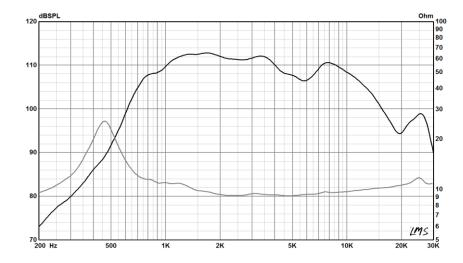
Frequency response and impedance of 1225-16 on specified horn, free field <sup>3</sup>.
