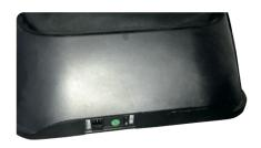
Make sure the plug is fully inserted in the chair port. The power line must remain untangled to avoid damage.
