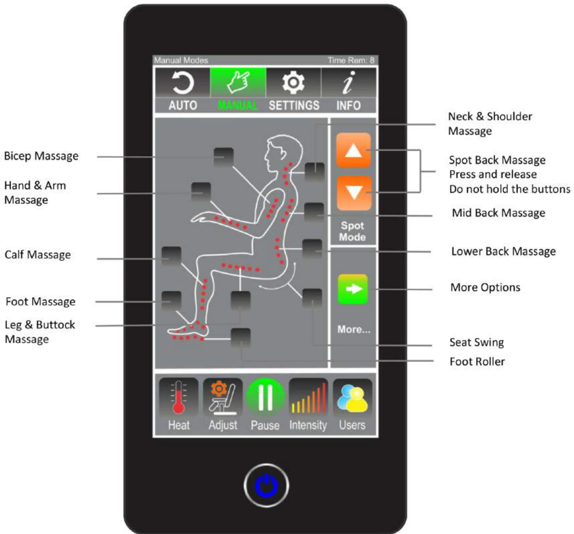
Fig.10: Manual Mode Descriptions
