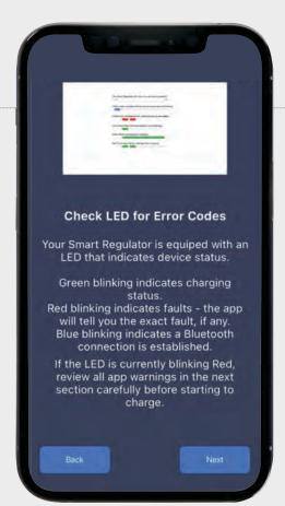
There is an LED light near the ports on your regulator. If the LED is currently blinking red, review all of the app warnings in the next section.
