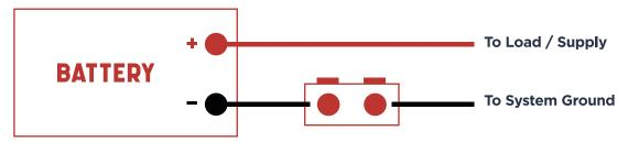
Positive side shunts are typically used with case ground alternators.
