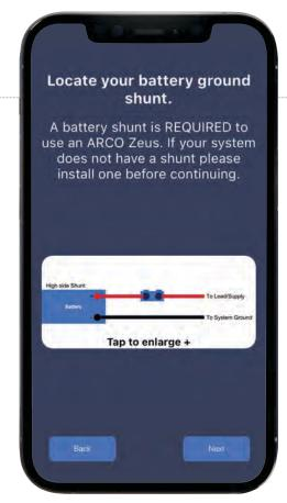
A battery shunt is required to observe current limitations for the battery bank in addition to the use of the onboard battery monitor.
