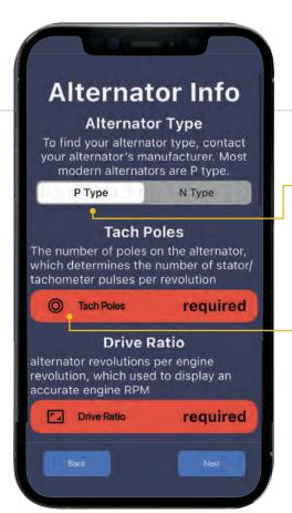
To find your alternator type, contact your alternator's manufacturer. **Most modern alternators are P type.**
