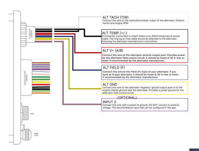
Follow your alternator wiring harness connections carefully. The wiring harness instructions are included within this manual and can also be enlarged in the app by long pressing the wiring harness instruction image.
