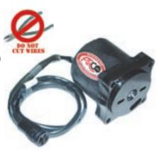
**6239** (NEW) **HEAVY-DUTY** FITS: HONDA 1992-2002 35-50 HP 2-wire connection Includes O-ring 4-bolt mount **Hollow-hex shaft** Female Spade Terminal Ends
