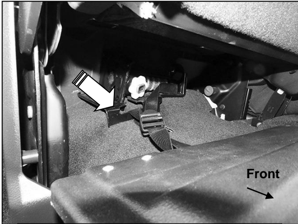
(Fig 5) Attach passenger/right Anchor Strap to jack mounting bracket (arrow)
