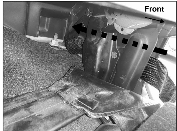
(Fig 2) Insert blank end of strap between inner and outer plates on driver/left side seat base. NOTE: Anchor Strap can also be wrapped around outside of seat base but is more visible
