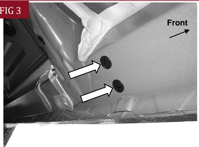
(Fig 3) Driver/Left center mounting location
