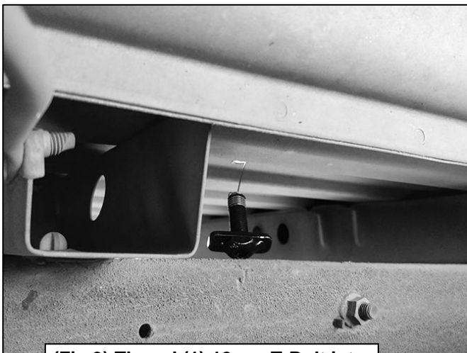
(Fig 3) Thread (1) 12mm T-Bolt into (1) 12mm Fish Wire. Slide the end of the Fish Wire into the drilled-out hole from the bottom of the bed
