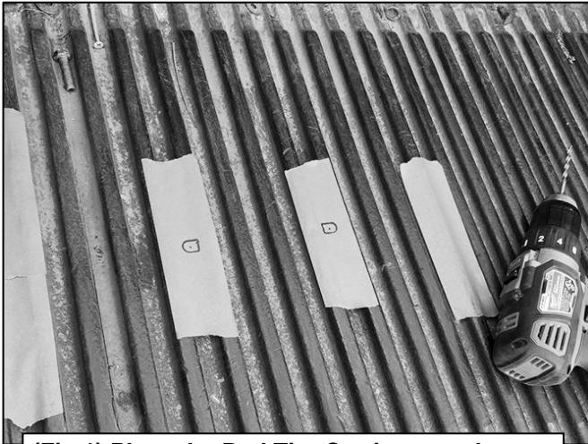
(Fig 1) Place the Bed Tire Carrier onto the desired location on the floor of the bed. Place tape onto the bed under slots. Mark locations for drilling. IMPORTANT: Check underneath the bed to avoid drilling through gas lines or other important fixtures under the bed.
