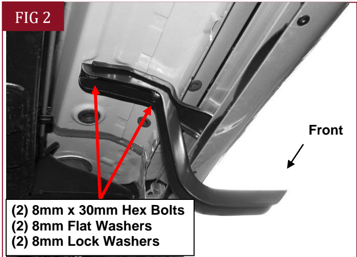
(Fig 2) Install the Mounting Brackets one at a time over the factory rocker panel brackets
