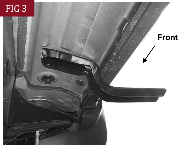
(Fig 3) Passenger/Right side Front Bracket attached
