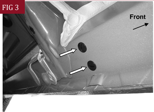
(Fig 3) Driver/Left center mounting location
