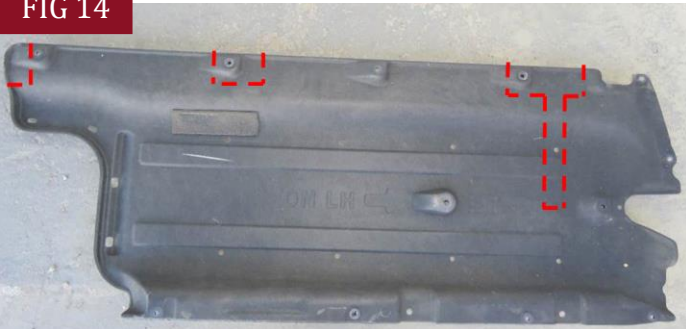
(Fig 14) Cut the plastic cover for Brackets clearance
