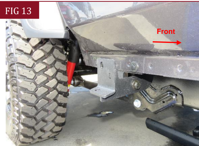
(Fig 13) Attach Passenger/Right Rear Bracket and Passenger/Right Rear Support Bracket to the rear location
