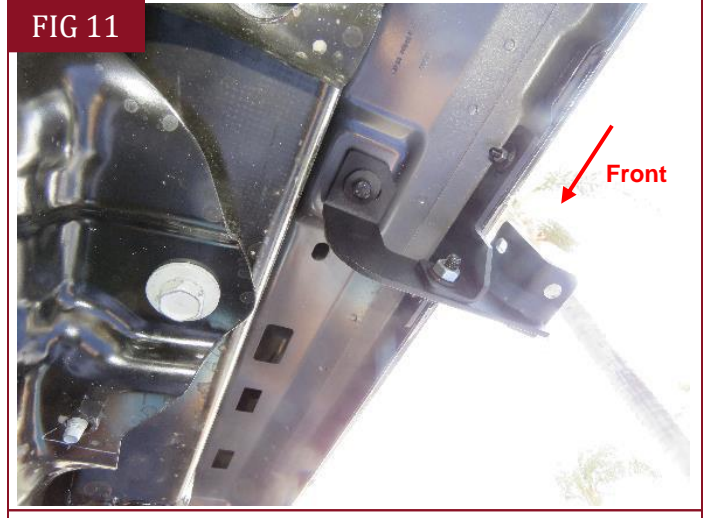
(Fig 11) Attach Passenger/Right Center Bracket and Passenger/Right Center Support Bracket to the center location
