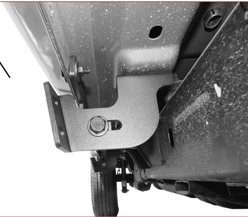
(Fig 7) (1) Passenger/Right Center/Rear Mounting Bracket and (1) Center Support Bracket attached to the 2nd location
