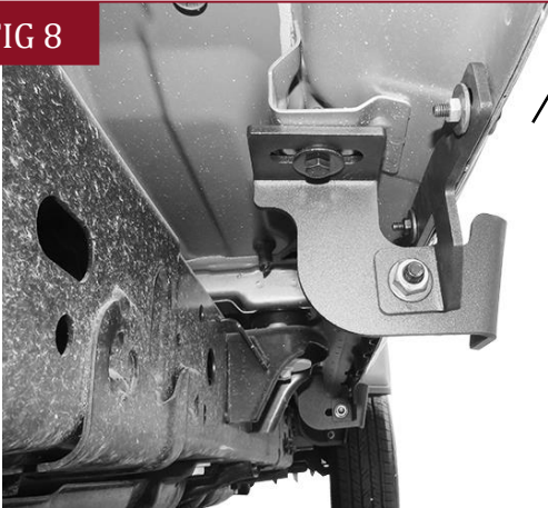
(Fig 8) (1) Passenger/Right Center/Rear Mounting Bracket and (1) Center Support Bracket attached to the 3rd location
