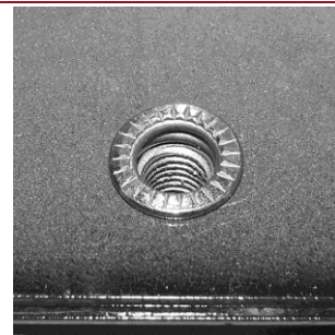
(Fig 15) Properly installed Insert
