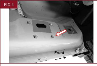
(Fig 4) Driver/Left side front mid 2015-on (example of models with factory installed threaded inserts)
