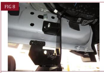
(Fig 8) Driver/Left Mounting Bracket and Support Bracket attached to the Front Mounting Location.
