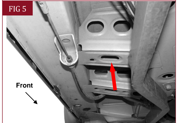
(Fig 5) Driver side center mounting location
