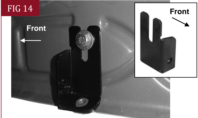
(Fig 14) Slide Upper Bracket over weld nut if equipped
