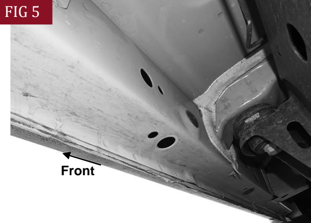
(Fig 5) Remove rubber plugs from the Passenger/Right center mounting location
