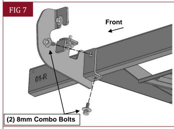
(Fig 7) Attach the Passenger/Right DS7 Running Board to the Mounting Brackets
