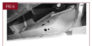
(Fig 6) Remove rubber plugs from the Passenger/Right rear mounting location
