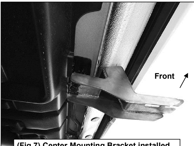
(Fig 7) Center Mounting Bracket installed
