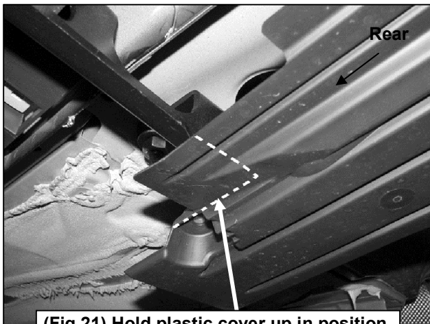
(Fig 21) Hold plastic cover up in position to determine area to cut from cover
