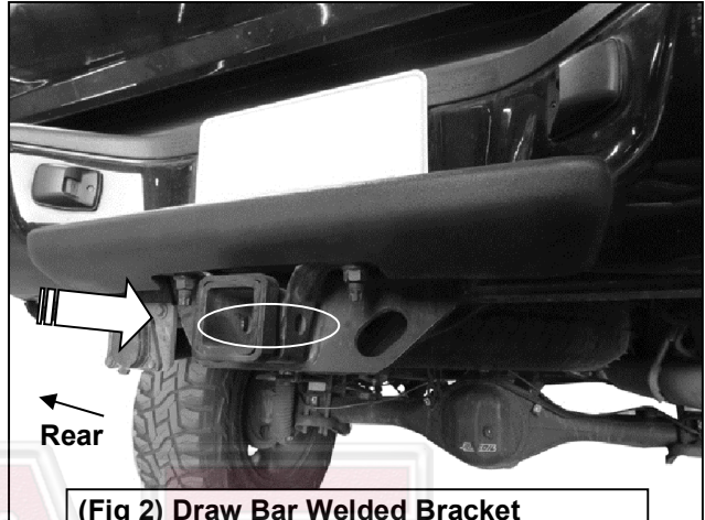
(Fig 2) Draw Bar Welded Bracket mounting location pictured
