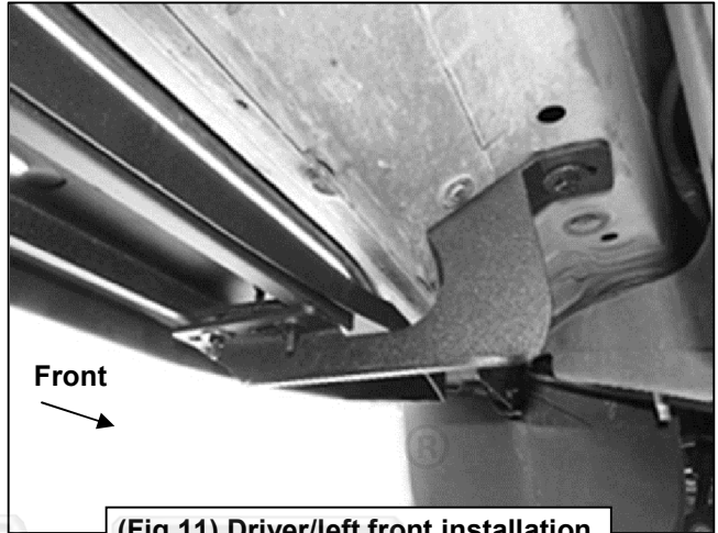
(Fig 11) Driver/left front installation
