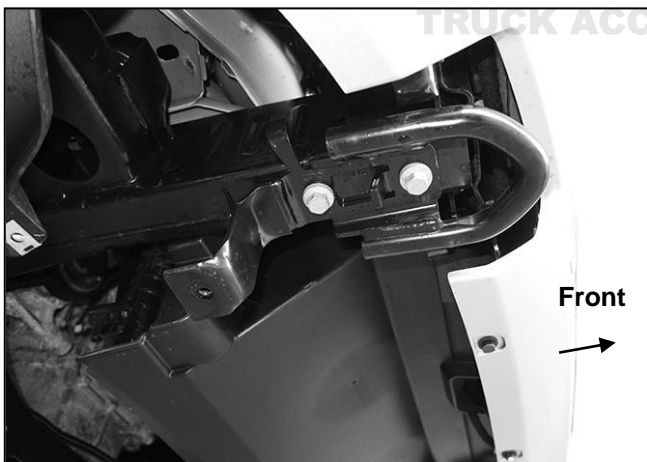
(Fig 3) Models with steel skid plate, temporarily remove skid plate to access tow hooks
