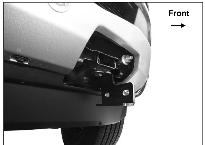
(Fig 8) Driver/left Frame Bracket installed on model equipped with tow hooks pictured
