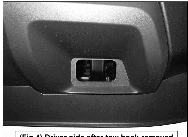
(Fig 4) Driver side after tow hook removed
