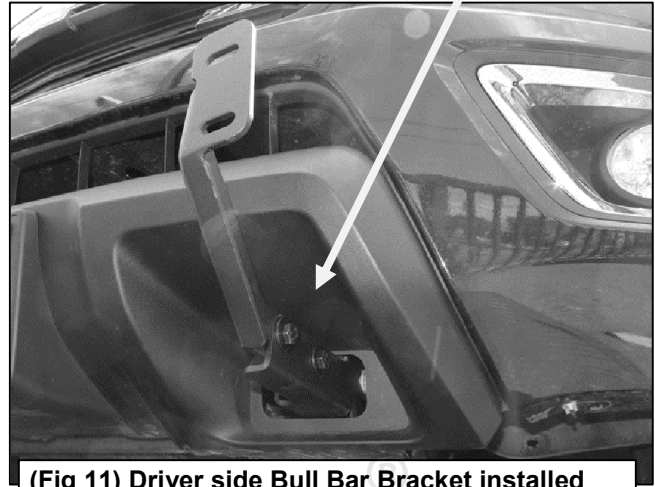
(Fig 11) Driver side Bull Bar Bracket installed
