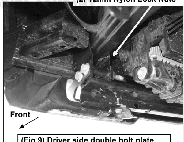
(Fig 9) Driver side double bolt plate pictured from behind bumper
