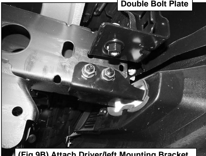
(Fig 9B) Attach Driver/left Mounting Bracket assembly to end of frame with Bolt Plates
