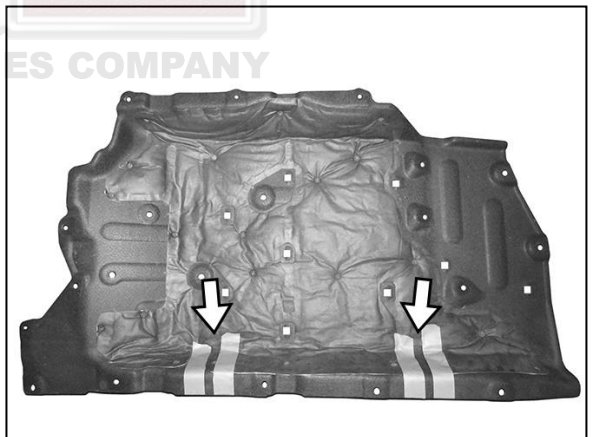
(Fig 16) Hold plastic cover up to bottom of Mounting Brackets to determine area to cut from cover. Use masking tape as a guide (arrows). Check for clearance after cutting and reinstall cover
