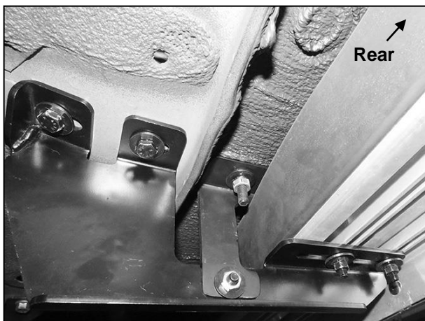
(Fig 12) Passenger/right rear Mounting Bracket and Support Bracket installed
