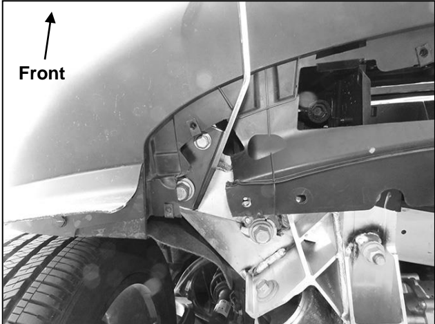
(Fig 4) Slide the inner slot end of the Bracket under the larger 21mm hex bolt. Reuse the 16mm hex bolt to attach Bracket
