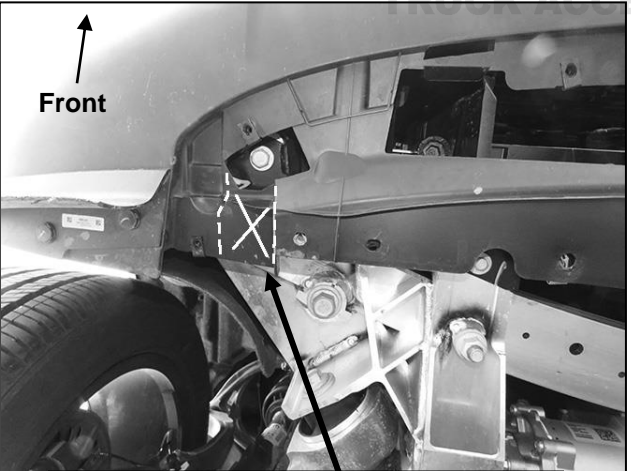
(Fig 3) Cut section from bumper cover to clear the Mounting Bracket
