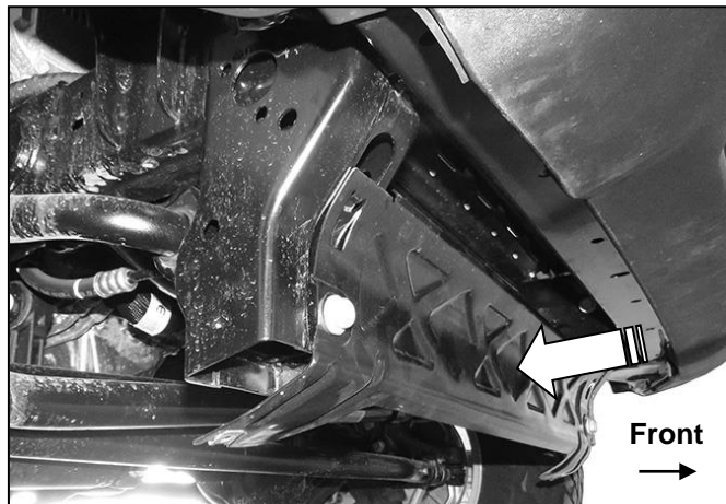
(Fig 1) Remove splash guard and bracket (arrow)
