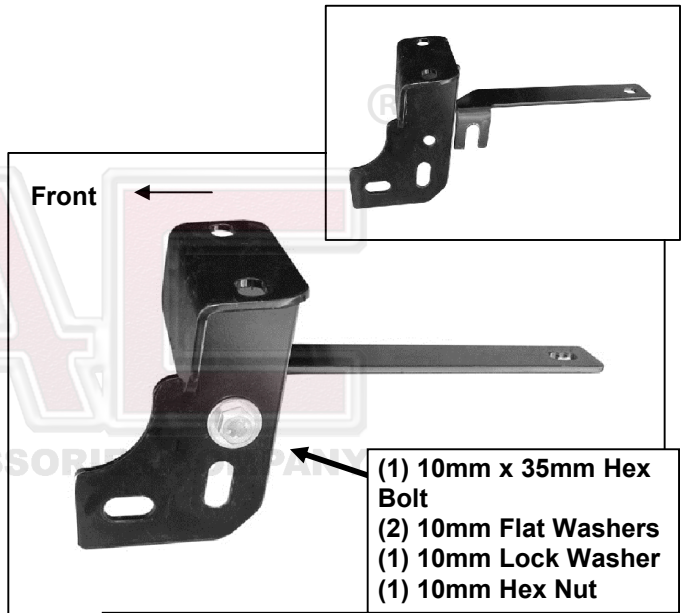
(Fig 3) Driver side Support Bracket in "no Tow Hook" position
