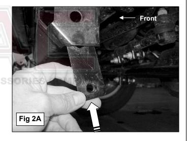
Insert the 12mm Double Nut Plate (2B) into the opening in the bottom of the end of the crossmember with the flat side against the crossmember (Fig 2A) and the hex nuts facing inward (Fig 2B)
