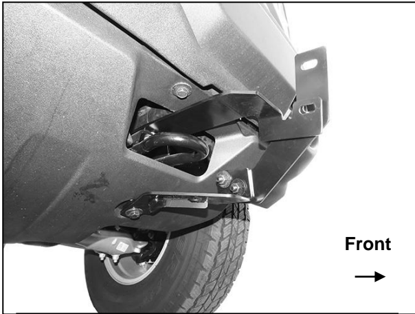
(Fig 11) Driver/left side Brackets installed
