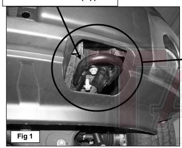
NOTE: On vehicles without tow hooks, the area circled above may be covered, (see Figure 4). Remove the lower plastic bumper cover to access the front of the frame channel for Bracket installation
