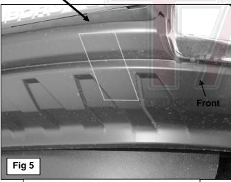
NOTE: Outline illustrated for example only. Only remove enough plastic for Bracket clearance. Do not cut through the front or rear edge of the cover.
