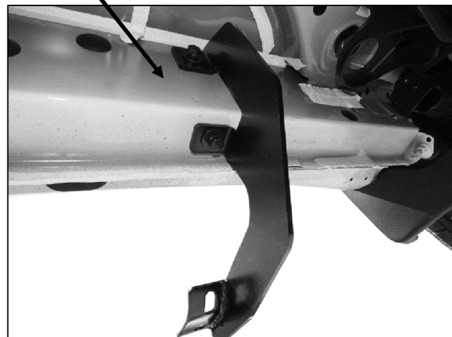
(Fig 4) Driver/left front Bracket installed
