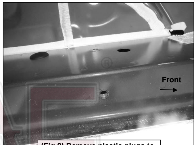
(Fig 2) Remove plastic plugs to uncover threaded inserts
