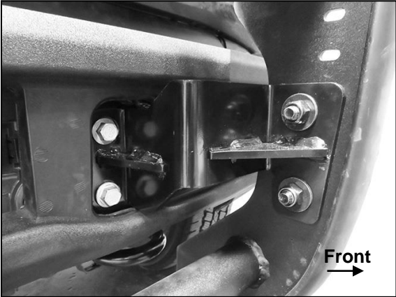
(Fig 23) Grille Guard assembly attached to outside of driver/left Mounting Bracket
