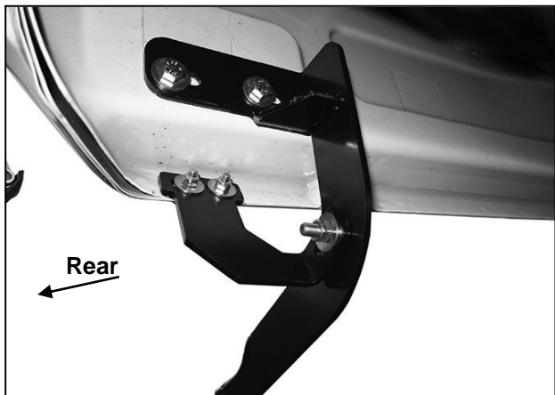
(Fig 16) Driver/Left rear Brackets installed
