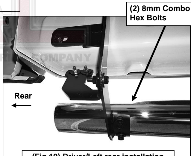
(Fig 19) Driver/Left rear installation
