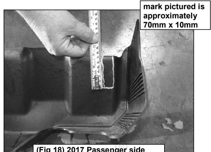
(Fig 18) 2017 Passenger side DEF cover marked for trimming
