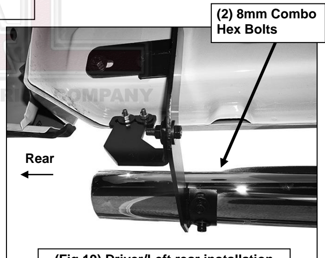
(Fig 19) Driver/Left rear installation
