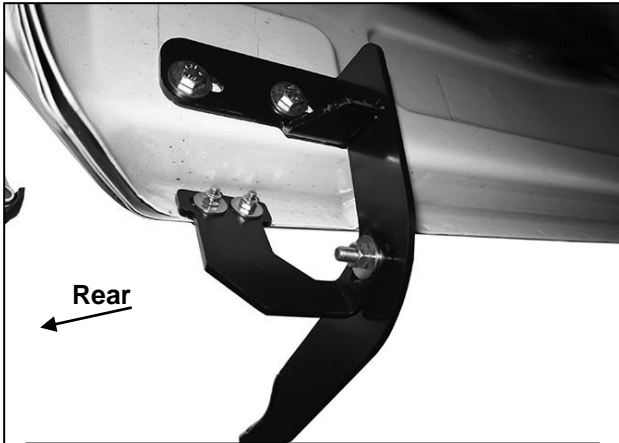
(Fig 16) Driver/Left rear Brackets installed
