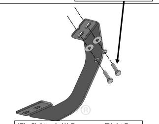
(Fig 5) Attach (1) Passenger/Right Rear Mounting Bracket to the 2nd location
