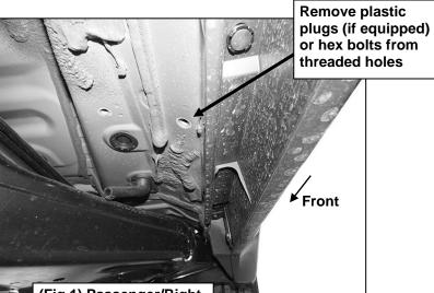
(Fig 1) Passenger/Right front mounting location
