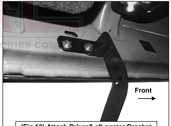
(Fig 13) Attach Driver/Left center Bracket
