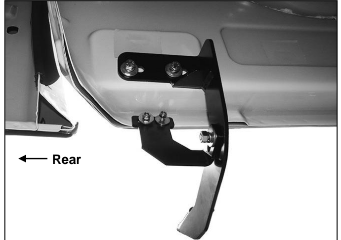
(Fig 16) Driver/Left rear Mounting Bracket assembly
